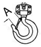
When measuring hook openings the use of vernier calipers is required. Any load chain that exceeds the maximum load chain dimensions shown above must be immediately replaced with new load chain
