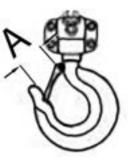
When measuring hook openings the use of vernier calipers is required. Any load chain that exceeds the maximum load chain dimensions shown above must be immediately replaced with new load chain
